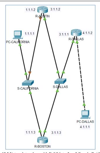
Figure 13.3 Network topology with Fa0/0 interface failure in R-AUSTIN
