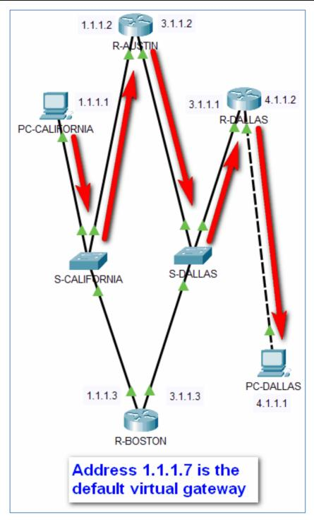
Figure 13.10 Route in case of failure R-BOSTON
