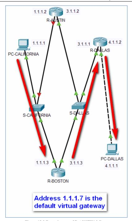
Figure 13.9 Route in case of R-AUSTIN failure
