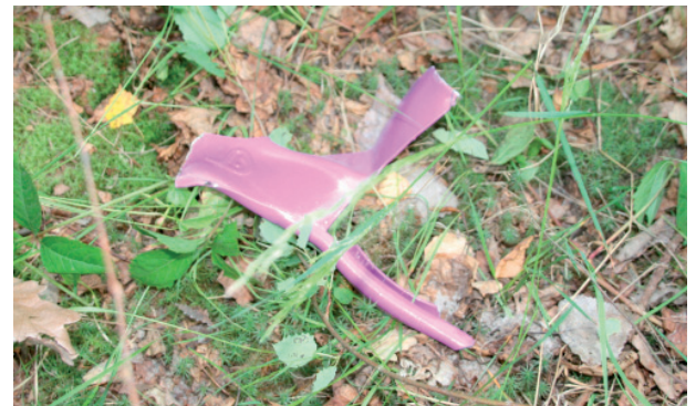
Fig. 6. Safety collar after explosion.
