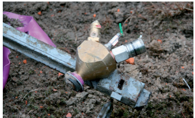
Fig. 5. Gas cylinder top with sensor outlet after explosion.
