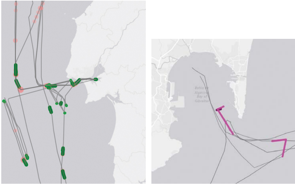
Figure 6.10. Trajectories with marked angle anomalies. Left: anomalies on straight trajectories. Right: false positives around ports
