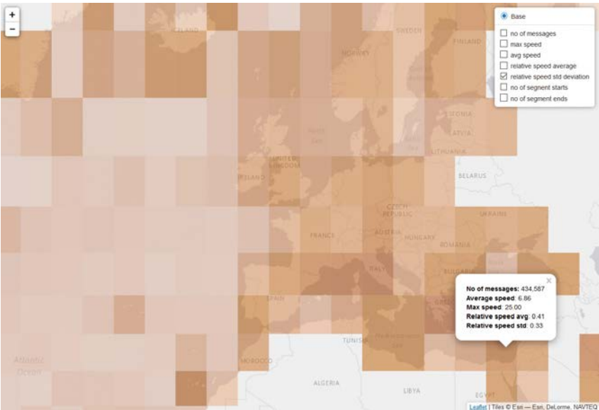
Figure 6.6. Standard deviation of the relative speed of vessels in a given segment, Europe
